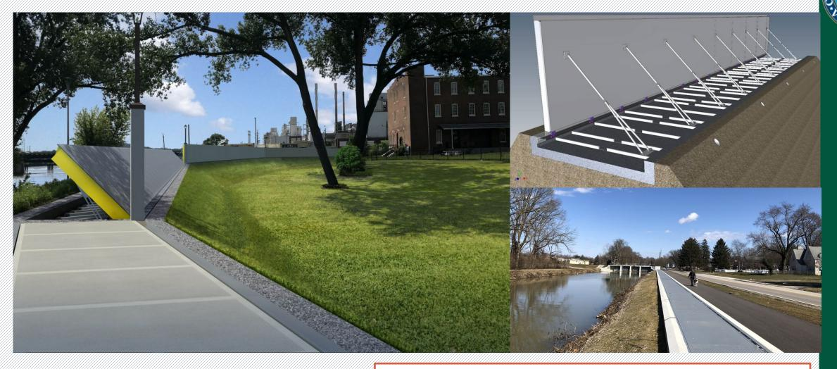
To install product along the entire bulkhead, material cost is ESTIMATEd to be ~\$5M for a 3.5-ft self-deploying wall.
