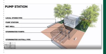
Requires new/larger inlet structures, new/larger storm sewer pipes, and pumping.
